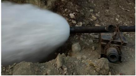
Geothermal water contains very less CO2 and H2S. It is not corrosive. TDS value is 3822 mg/l at first well. Electrical submersible pumps are installed at 490-600 m depth with 155 °C temperature (each 240-350 tons/h).
